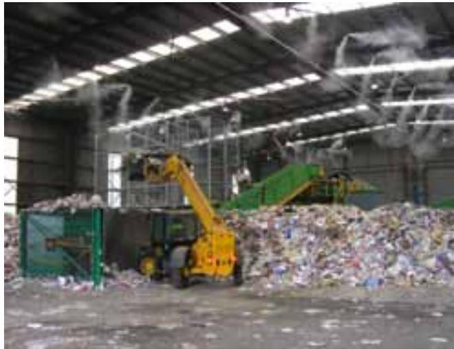
Overhead misting system in operation At Recycling Centre
